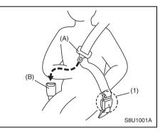
Before fastening the rear center belt, push the connector latch plate (1) at the end of the safety belt strap into the connector and make sure the webbing is not twisted. To fasten the belt, sit up straight and well back in the seat, pull the latch plate (A) across your body and press it into the buckle (B) until you hear a "click".
